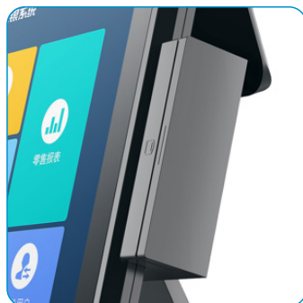
MSR port with connector Do not need to open the maincase to connect
