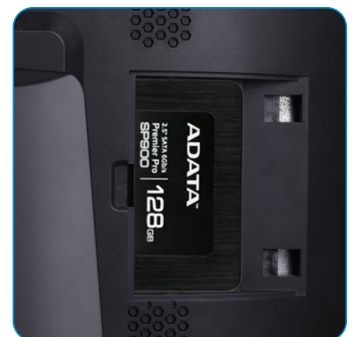
Port for SSD installation
